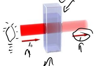
**Transmittance:** is the fraction of incident light that passes through a sample.
