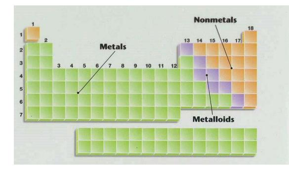
**Metals** – luster, high electrical and thermal conductivity, ductile and malleable.
