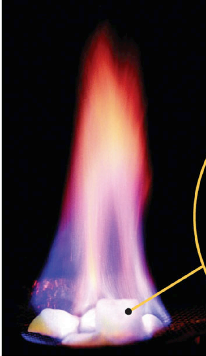
(a) Methane hydrate burns as methane gas escapes from the solid hydrate.
