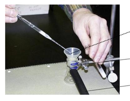
Transferring crystals with a pipet onto the filter paper on the Hirsch funnel.
