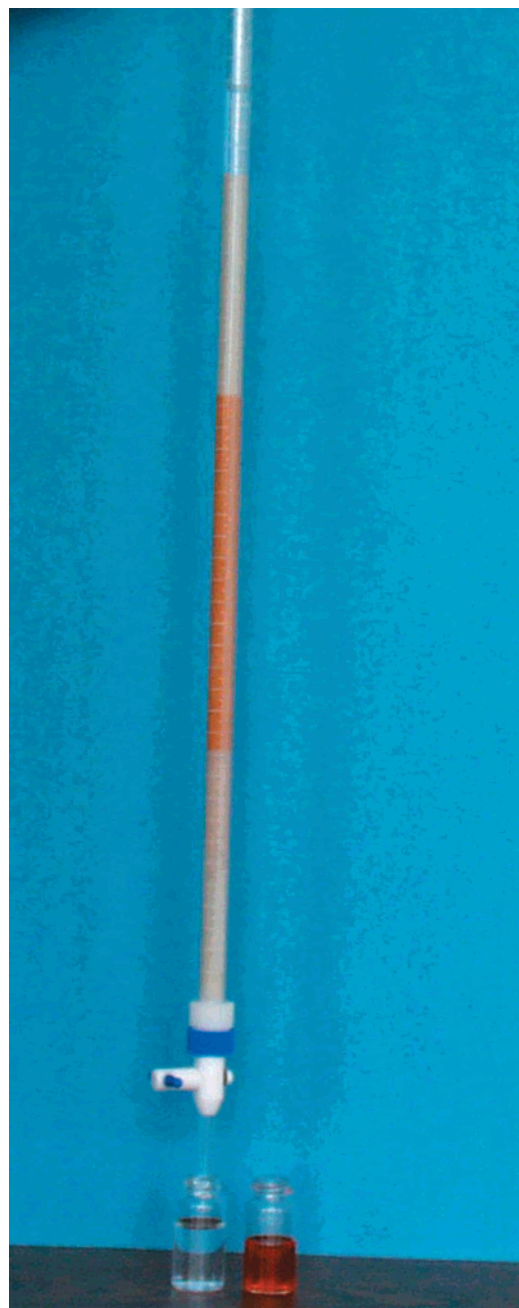
FIGURE 1. Trapping of an organic solution (Orange OT dye) onto polycation-micelle-treated sand.
