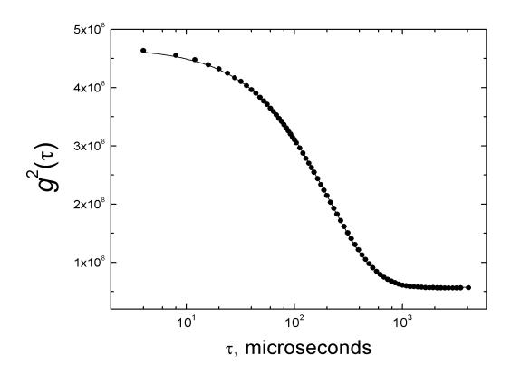
These data may not appear to decay exponentially; that is a result of the log scale on the  $\tau$  axis, which expands the range for small values of  $\tau$ .
