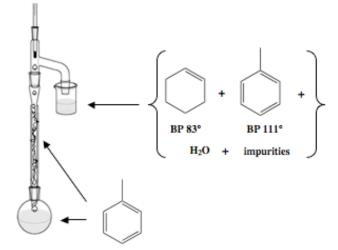
Once the toluene distills up the column and reaches the thermometer, most of the cyclohexene and water has been pushed over into the collection vial along with some toluene. The distilling flask contains phosphoric acid, toluene, and higher-boiling impurities. The column contains mostly toluene.
