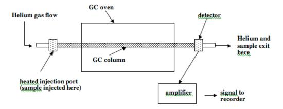
A very small sample (  $\sim 0.1 \,\mu l = 0.0001 \,m l$ ) is injected into the hot injector port.
