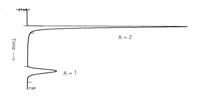
The injection point is at "start" at the top of the chromatogram. The peak labeled "A = 2" is due to the low-boiling liquid which reaches the detector first. The peak labeled "A = 1" is due to the high-boiling liquid which reaches the detector later.
