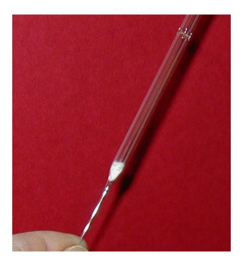
Scoop up some silica gel into the wide end of the pipet, turn the pipet upright, and tap the pipet gently so that the silica gel packs evenly down into the small end. Continue adding silica gel until the pipet is about half full.
