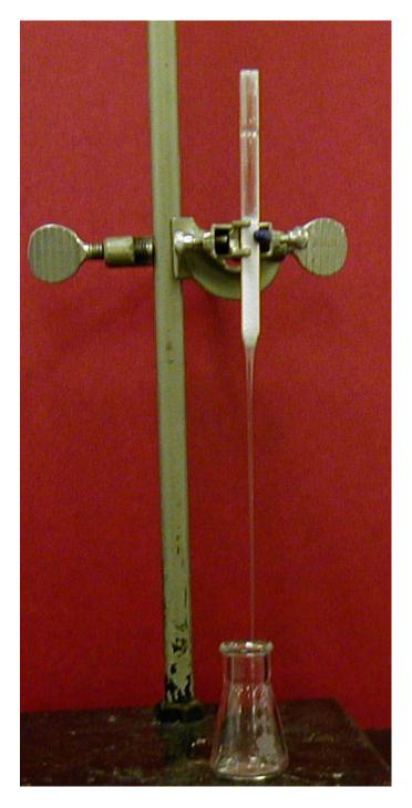
Add about 1 mL of ligroin to the top of the column and allow it to drain through the column into a small Erlenmeyer flask. It will take a few minutes for the ligroin to pass through the column and begin to drain. If draining is too slow it may be that the cotton was packed too tightly. What
