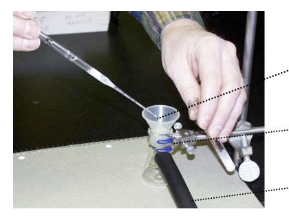
Transferring crystals with a pipet onto the filter paper on the Hirsch funnel.
