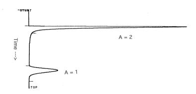
The injection point is at "start" at the top of the chromatogram. The peak labeled "A = 2" is due to the low-boiling liquid which reaches the detector first. The peak labeled "A = 1" is due to the high-boiling liquid which reaches the detector later.
