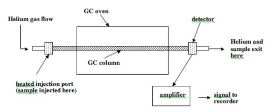
Schematic of a Gas Chromatograph
