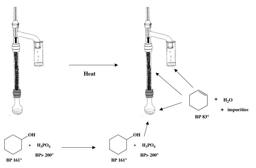
Cyclohexanol plus Phosphoric Acid are heated As the reaction proceeds, cyclohexanol is being converted to cyclohexene and water (plus some impurities). The low-boiling cyclohexene and water boil at the high temperatures and distill up the column and into the collection vial. As with all distillations though some is left behind in the flask and in the column.
