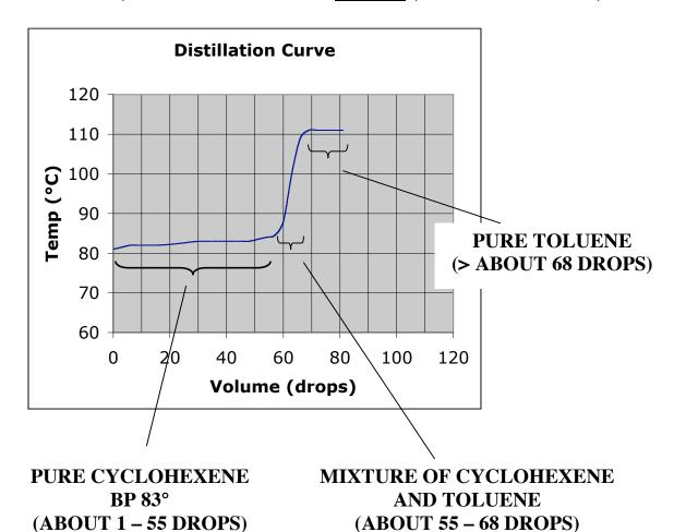
LIQUID THAT DISTILLS BELOW THE 83° PLATEAU (< ABOUT 81°) IS CONSIDERED TO BE LOW-BOILING IMPURITY.
