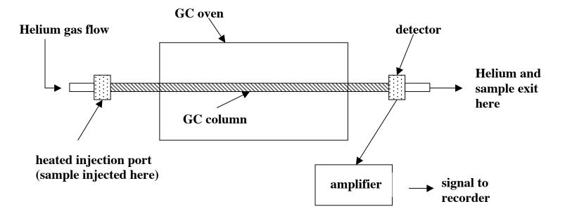
INJECT SMALL SAMPLE ( ~ 0.1  $\mu$ L = 0.0001 mL) INTO HOT INJECTOR PORT.
