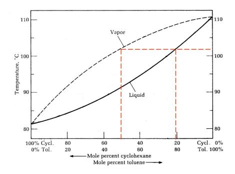
WHAT RESULTS IN DOING ONE VAPORIZATION-CONDENSATION STEP STARTING WITH A MIXTURE OF 20% CYCLOHEXANE AND 80% TOLUENE?
