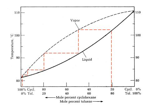
WHAT RESULTS IN DOING FOUR VAPORIZATION-CONDENSATION STEPS IN ONE PROCESS, STARTING WITH A MIXTURE OF 20% CYCLOHEXANE AND 80% TOLUENE?
