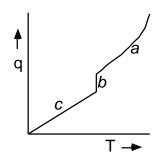
For region (a) of the process, you can discern that the heat capacity ( $C_p$ ) is (**zero** / **non-zero**).
