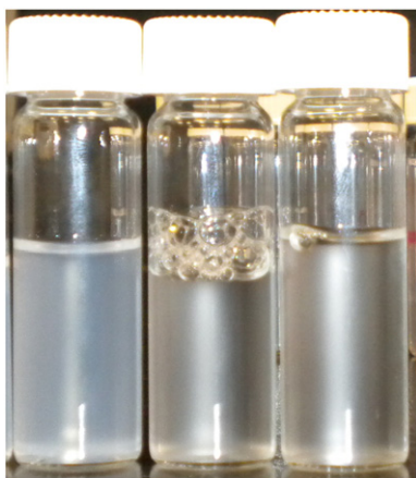
Fig. 1. Typical coacervate suspensions (before centrifugation) of poly(dimethyldiallyl-ammonium chloride) (PDADMAC)/sodium dodecyl sulfate (SDS)-Triton X-100, at Y = 0.4 , I = 0.4 M NaCl (see Section 2.1).
