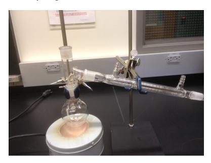
4. Attach a condenser adaptor to the end of the condenser and hold it on with an elastic band. Connect rubber tubing to the condenser and attach the lower connection to the water source and the upper one to the drain. Start a slow flow of water through the condenser.
