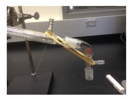
5. Carefully place a thermometer into the thermometer adaptor and set it into the apparatus. Place a receiving flask under the condenser adaptor to collect the distillate. Move the ring and heating mantle up to the flask to make contact. Have your TA check things out then do the distillation.
